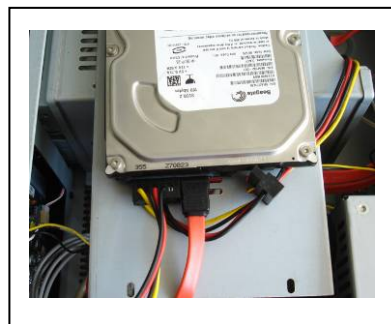
2. Connet power and data cable.
