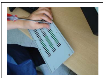
1. Fix the HDD on the bracket.
