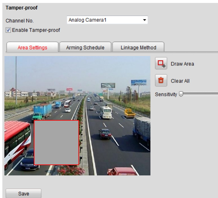
Figure 7.22 Tamper-proof Alarm Settings
