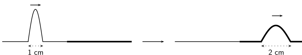
Figure 5.7: Reflection and transmission of a pulse at the boundary between two media.
